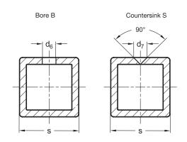
The square dimensions of the locking slide units are designed for construction tubes GN 990. These can be fitted with locking holes (B or S) by the user according to the dimensions specified in the table.
