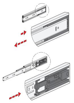
Telescopic slides GN 1418 come with a "push to open" or "touch to open" mechanism. In addition to ease of opening, the system allows you to have drawers without a front handle. The visual appearance is trim and high-end.
