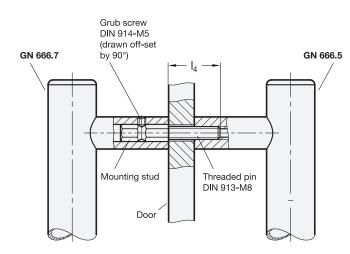
Tubular handles GN 666.5 / GN 666.7 allow the mounting of a pair of handles in opposite position. This method could be used on doors (double handle).
