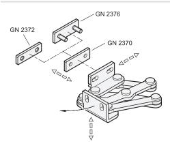
The multiple-joint hinges can be adjusted in three planes during installation. For example, this allows tolerances to be adjusted or the required compressive forces for seals to be established. Two planes can be adjusted via the parallel or perpendicular slots in the fixing angle pieces. In the third plane, position corrections can be made using the spacer plates GN 2370.
