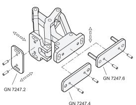
The multiple-joint hinges can be adjusted in three planes during installation. For example, this allows adjustment for tolerances or establishing of required compressive forces for seals. Two planes can be adjusted via parallel or perpendicular slots in the fastening flanges. In the third plane, position corrections can be made using the spacer plates GN 7247.2.
