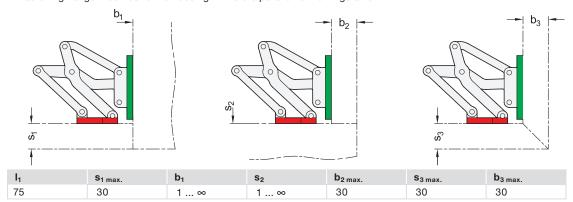
2. Fastening flange mounted to the housing with slots perpendicular to the hinge axis:
