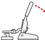
Moving the lever arm back will lift the latch bolt and release the catch (one-hand operation).
