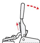
The latch bolt engages with the catch if the locking mechanism is moved upward during clamping.
