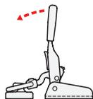
For **clamping**, lift the lever arm until the latch bolt rests against the catch.
