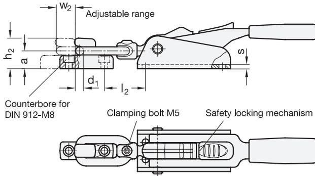
Dimensions of installation (Top view)
