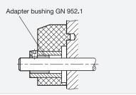
**Clamping plates GN 955.6** (→ *Page XYZ*) can be used to clamp spindles after adjustment to secure them against independent or accidental turning.
