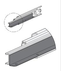
Support brackets on the inner slide are available on request for some slide variants, even in small quantities. The support bracket is used for simple mounting, for example, of a drawer, if side mounting is not possible. Mounting occurs by means of through-holes that are arranged at a right angle in the bracket.
