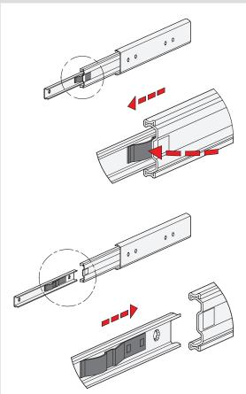
Telescopic slides with a detach function can be completely separated from one another in the area of the middle and inner slide. This feature not only facilitates mounting. It also allows the extension to be quickly removed, for example, when maintenance work is performed on the components located behind.
