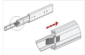
The locking function is noticeable by a slight resistance of the slides in the end positions, which has to be overcome on opening and closing. The locking device in the back stop position is usually integrated into the rubber stop function, making additional components unneces-
