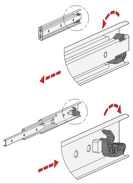
Telescopic slides can have an integrated self-retracting mechanism, which improves considerably the ease of use when closing the extensions.
