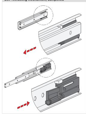
Dampened self-retracting mechanisms are also called "soft-close" and are divided into two main functions. They offer the best possible ease of use on closing the
