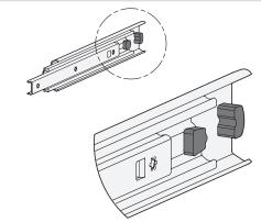
The rubber stops used in almost all slide variants dampen the impact of the slide in the respective end position. This feature minimizes noise development and increases the lifespan. Attached to the slides in a partially concealed, partially visible manner, the stops meet each of the requirements in regard to shape, material, and hardness.
