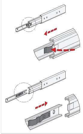
Telescopic slides with a detach function can be completely separated from one another in the area of the middle and inner slide. This feature not only facilitates mounting. It also allows the extension to be quickly removed, for example, when maintenance work is performed on the components located behind.
