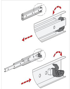
Telescopic slides can have an integrated self-retracting mechanism, which improves considerably the ease of use when closing the extensions.
