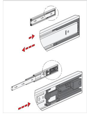
Telescopic slides can be fitted with a "push to open" or "touch to open" mechanism. In addition to ease of opening, the system allows you to have drawers without a front handle. This makes it easy to achieve a sleek, highend appearance.
