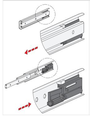
Dampened self-retracting mechanisms are also called "soft-close" and are divided into two main functions. They offer the best possible ease of use on closing the extension.
