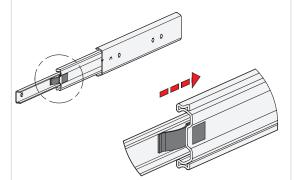
The locking function is noticeable by a slight resistance of the slides in the end positions, which has to be overcome on opening and closing. The locking device in the back stop position is usually integrated into the rubber stop function, making additional components unnecessary.
