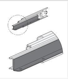
Support brackets on the inner slide are available on request for some slide variants, even in small quantities. The support bracket is used for simple fastening, for example, of a drawer, if side mounting is not possible. Fastening occurs by means of through-holes that are arranged at a right angle in the bracket.
