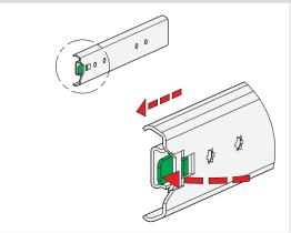
Unlike locking devices, a latch secures the slides in the stop positions in a frictionally engaged way. Telescopic slides with latches are used when the slides need to be protected against independent extension or retraction, for example, due to a tilted position.
