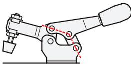
Even the slightest forward movement of the operating lever brings the clamping arm with the contact pad over the workpiece.
