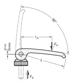
The eccentric principle has two advantages: A large clamping force  $F_S$  and a self-locking mechanism as soon as the dead centre is exceeded.
