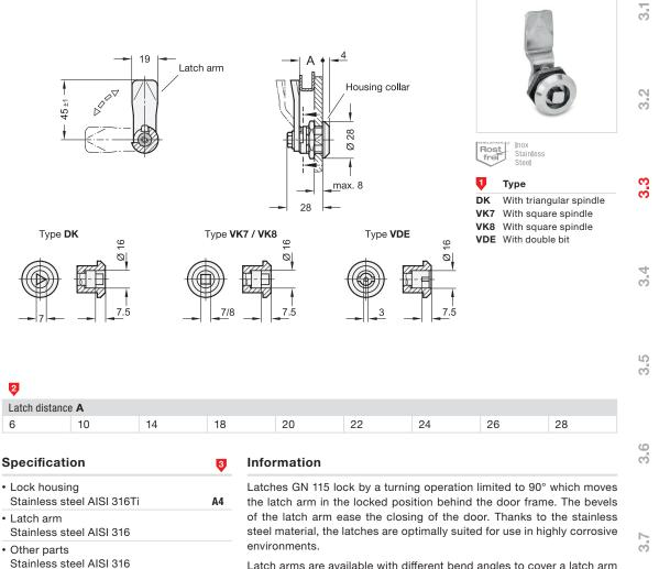
Latch arms are available with different bend angles to cover a latch arm distance A from 6 to 28 mm.
