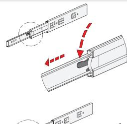
Type F has additionally a detach function through which the extension slides can be completely separated from one another in the area of the middle and inner slide. This feature not only facilitates mounting. It also allows the extension to be quickly removed, for example, when frequent maintenance work is performed on the components located behind.
