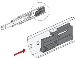
Telescopic slides GN 1424 have a dampened self-retracting mechanism, which is also called "soft-close". The dampened self-retracting mechanism is divided into two main functions and offers the best possible ease of use on closing the extension.
