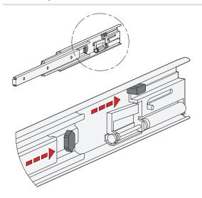
The rubber stops of type B dampen the impact of the slide in the respective end position. This feature minimizes noise development and increases the lifespan. Attached to the slides in a partially concealed, partially visible manner, the stops meet each of the requirements in regard to shape, material, and hardness.
