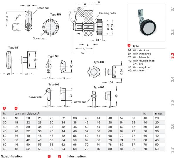
Lock housing Zinc die casting Housing collar
