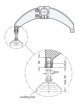
The adjustment or leveling feet are installed as shown in the outline. The maximum projection of the leveling feet must not be exceeded.
