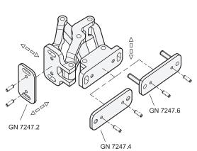
The multiple-joint hinges can be adjusted in three planes during installation. For example, this allows adjustment for tolerances or establishing of required compressive forces for seals. Two planes can be adjusted via parallel or perpendicular slots in the fastening flanges. In the third plane, position corrections can be made using the spacer plates
