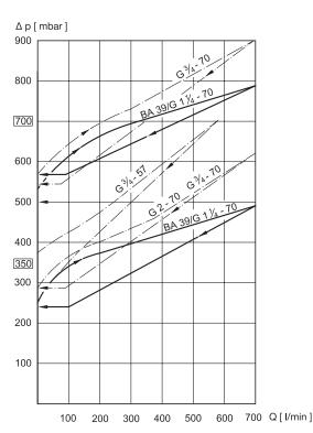
Pressure curve  $\Delta p$  [mbar] in the container as factor of the air flow rate [l/min.] at a valve opening pressure of 350 or 700 mbar.
