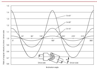
The single universal joints transfer the initial steady rotation as an irregular rotation because one revolution of the drive shaft using the single universal joint will cause the driven shaft to accelerate and decelerate twice. The extent of the irregularity depends on the operating angle 8.
