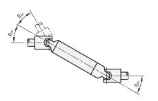
For a steady transfer of rotation, the inclination angles B must be equal on both ends of the connecting shaft.
