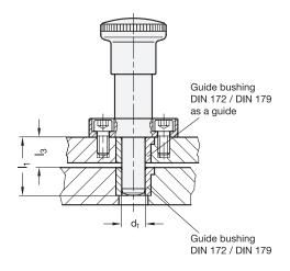
Two different plunger pin lengths I<sub>1</sub> are available for each indexing plunger diameter d<sub>1</sub>.
