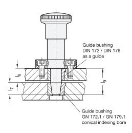
The length I<sub>7</sub> is determined by the penetration depth of the plunger pin into the cone of the bushing.
