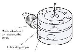
Screw for additional clamping of the rotary disk
