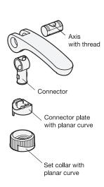
$\mathbf{I}_{\!\scriptscriptstyle 4}$  adjustable by the set collar for optimum clamping force and covenient lever position.
