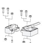
Prior to installation remove the slam latch cover as shown in the sketch. Socket cap screws DIN 912, hex head screws DIN 933 and hex nuts ISO 4032 each with thread size M 6 can be used for mounting the slam latch.
