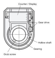
The transmission ratio and counting direction of the counter are determined by the pitch of the adjusting spindle. The indicated value after one turn starting from the 0 position serves as a characteristic value. Decimal places are indicated in red.
