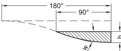
Looking at the developed view arising in an eccentric through the rolling motion, one will find that this is caused by a sinusoidal curve.
