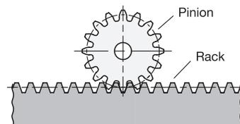
The most important mechanical value for the toothed racks is the maximum force that can be exerted on an individual tooth.
