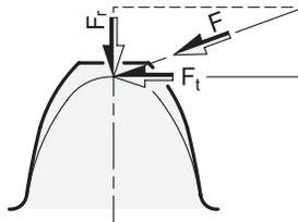
The tangential force  $F_t$  is then correlated with the torque via the pitch circle diameter. The following formula applies to the nominal torque:
