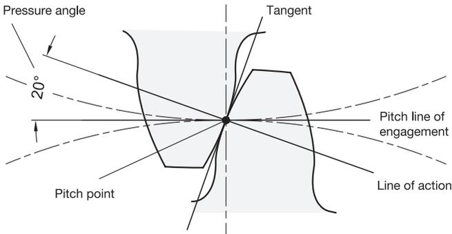
The tooth flanks of the gears are shaped as involutes.
